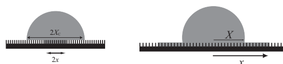
Fig. 2. (a) Mushroom state: x is the radius of the “nucleus”, and X is the radius of the contact circle. (b) Sunny-side-up state: x is the radius of penetration, and X is the radius of contact circle. X in the sunny-side-up state will be called the yolk radius.
